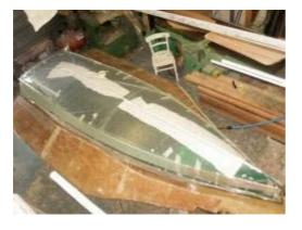
consolidate the laminate while it is curing and to soak up excess resin. To do this on top of the materials you need for the hull you will also need a vacuum pump and vacuum consumables which include the bag, peel ply, bleeder cloth and release film. You can expect to get a pump for about £50 second hand and £250 new and the vacuum consumables are likely to set you back about £
