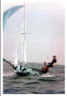
In 1991 the class adopted the Asymmetric spinnaker and this combined with new construction techniques lead to a bit of a building boom. The majority of boats built during this time were constructed Foam Sandwich largely in glass but with
