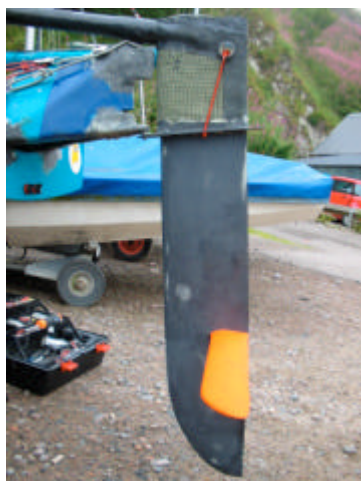
High aspect ratio foil used on AquaMarina and similar to that used on Primal Scream. Moving the stock changes the angle of attack.
