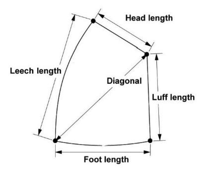
**Mainsail Rounds** – to be measured at the widest point, perpendicular to the straight line between two corners
