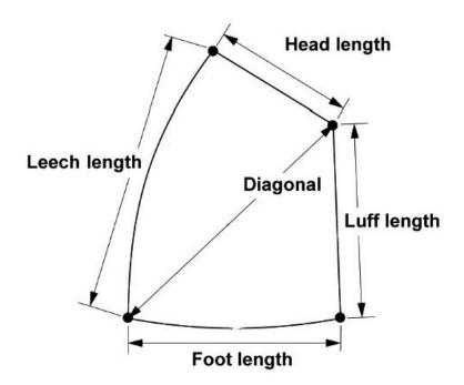
**Jib Rounds** – to be measured at the widest point, perpendicular to the straight line between two corners
